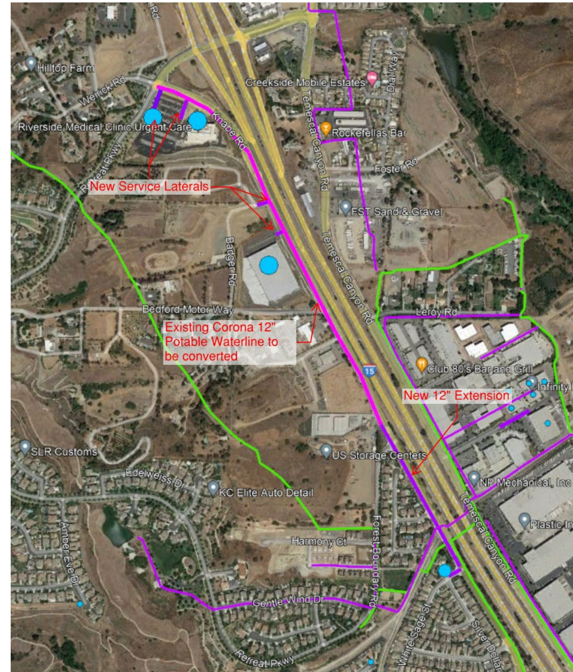
Project 2 Medical Center Corona/TVWD Recycled Water Pipeline
